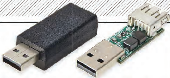
ABOVE: The JitterBug is a purely passive device (drawing no power from the USB hub) but provides transformer-isolation and RF filtering of both the 5V USB 'VBUS' and its differential data lines. Two JitterBugs may be used in parallel if necessary
