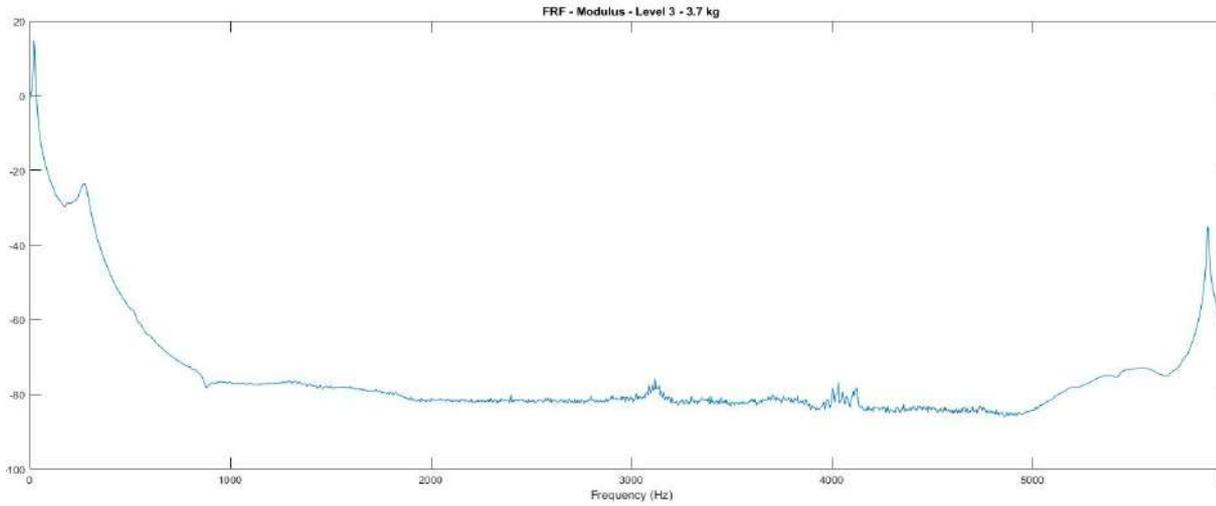
**Figure 9. FRF on Level 3 damper loaded with 3.7 kg.**
