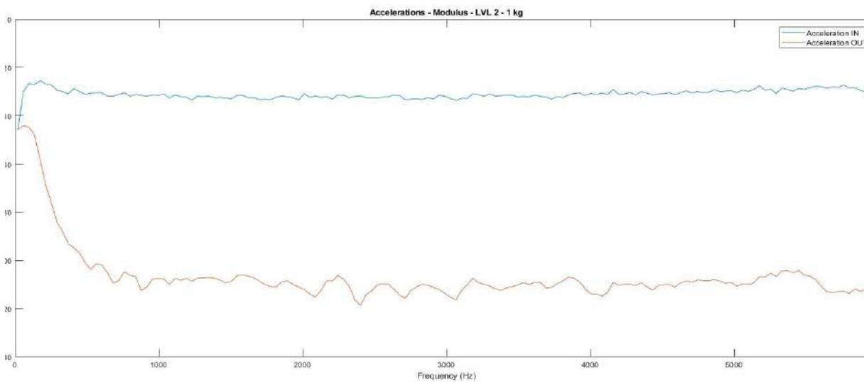
Figure 4. Incoming and outgoing accelerations on Level 2 damper loaded with 1 kg.
