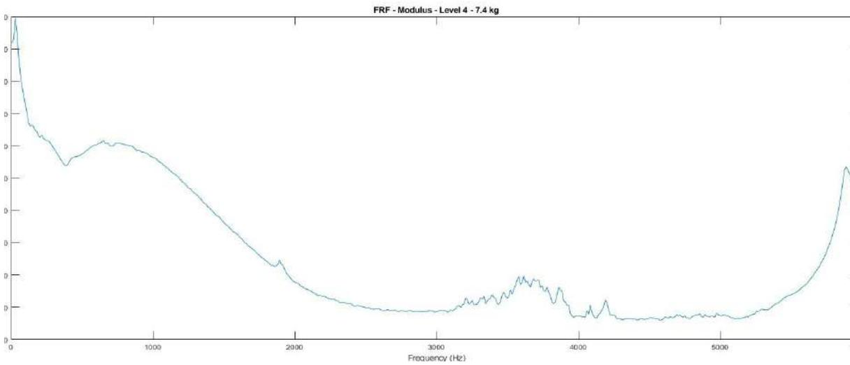
**Figure 10. FRF on Level 4 damper loaded with 7.4 kg.**
