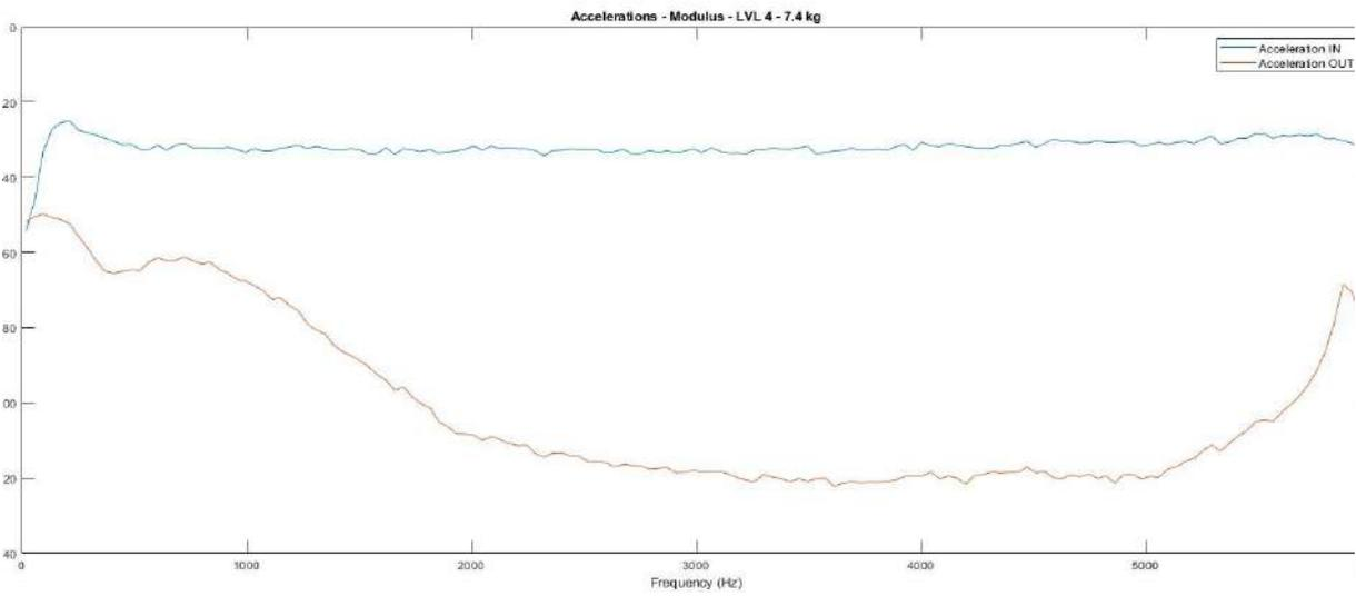
Figure 6. Incoming and outgoing accelerations on Level 4 damper loaded with 7.4 kg.
