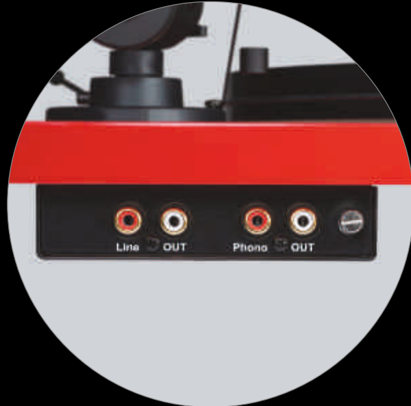
switchable line or phono output and built-in Bluetooth transmitter
