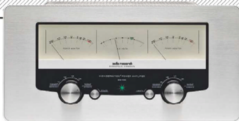
ABOVE: Dominating but also graceful, ARC's trio of analogue meters conveys a measure of mains line voltage, tube bias current (in adjustment mode) and power output. The log scaling of the latter seems of decorative value only as a sustained 10W/8ohm registered just '0.015' on the display
