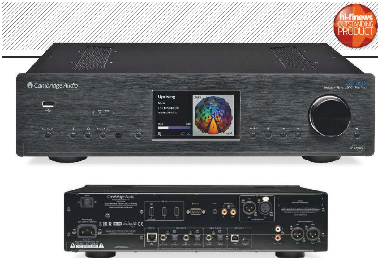
ABOVE: Four S/PDIF inputs and two outputs, one AES/EBU in and out, asynchronous USB-B, four USB-A (including an iDevice-compatible USB-A on the fascia), trigger, external IR and RS232. Analogue outs (fixed and variable) via RCA and balanced XLRs
