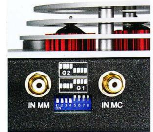
Each channel is equipped with dip switches to set G1 or G2 levels of gain.
