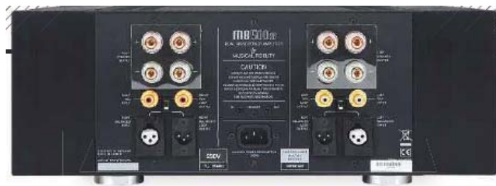
ABOVE: M8500s has two sets of speaker binding posts for bi-wiring and XLR and RCA loop-through sockets for easy bi-amping. 12V trig in/out sockets are also provided
