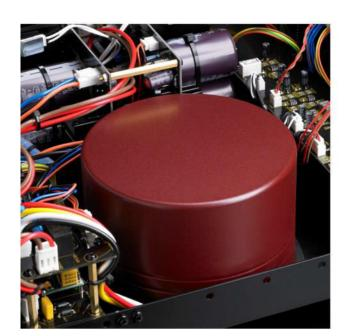
The heart of the HINT 6's power supply is a massive 1.1 kVA toroid power transformer. It is custom designed for well-contained radiated hum, high efficiency, and high power. Encapsulating this massive power transformer in an epoxy-filled steel canister assures ultra-quiet performance.
