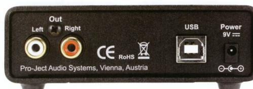
As simple as can be! The rear panel of the Pro-Ject USB Box S+ features a single USB input together with unbalanced RCA output jacks. Power comes from a standard 9V wall-wart.
