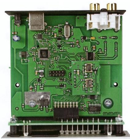
Inside the Pro-Ject uses an XMOS chipset and PCM5102A Burr-Brown DAC to handle digital duties. LED indicators at the front of the unit show sampling rate of incoming music files.
