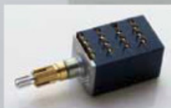
Custom-made 2-axis 4-gang volume controller
